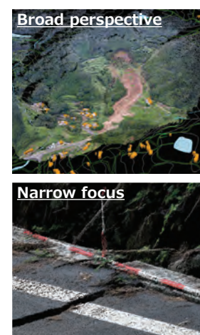
Figure1. Virtual disaster site using point cloud
