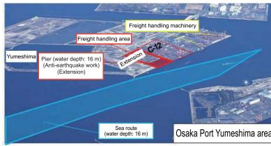
To enable large vessels operating on major sea routes to enter Kobe Port and Osaka Port, construction of large container terminals with global standard water depth and area is being promoted.
